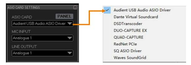
The AEQ function needs to call the ASIO driver of the sound card. When the ASIO driver is installed correctly on the computer, the PC software will automatically detect the ASIO sound card device, and then select the corresponding sound card.
