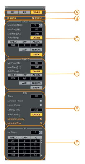
**A\_ MODE SWITCHING**: FIR/IIR/FIR+IIF optional, enabling FIR requires external EQ/Frequency division mode to use FIR filters (for example EQ mode: 17 PEQ+FIR can be used, 31 PEQ can not be used FIR).
