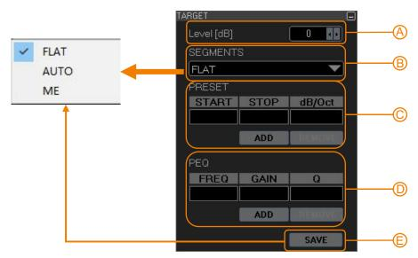
Target curve design, design the system target curve you want, and then generate the curve that fits the target through the AEQ operation to obtain the curve the user wants.
