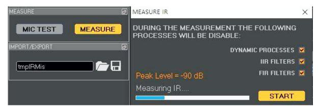
Click MEASURE to enter the measurement Click START to start the measurement, the blue progress bar ends and the measurement is completed
