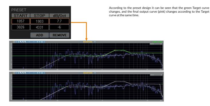
**D\_ PEQ:** Design the target curve in PEQ mode, when the current PEQ is selected, you can drag the drawing area to modify the frequency band and gain
