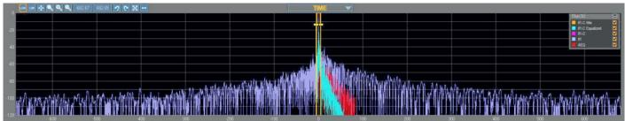
Used in conjunction with the time window, the range in the time window can be dragged and the impulse response can be manually windowed; the reflected sound pulse visible to the naked eye can be avoided, the accuracy can be improved and the reflected sound can also be taken into account as required. Non-experienced users can consider, use the automatic windowing function, and turn on AUTO WIN "ENABLE" to enable the automatic windowing process.
