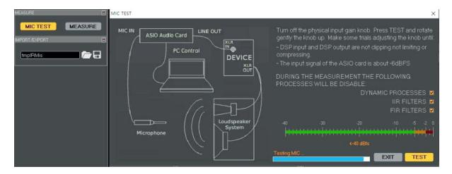
Select MIC TEST to test and adjust the output of the audio system and microphone acquisition; as setup, follow the simple diagram showing the right connection (the dynamic processes, IIR filter and FIR filter of the current channel will be disabled by default during the measurement process).
