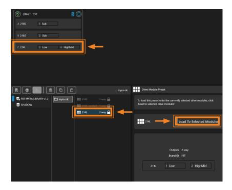
OUTPUT MATRIX setting is very important because it decides the number of ways assigned to a DSP channel and therefore the preset compatibility. The figure show the correct setting for AMP 1 where CH 1 & CH2 are assigned respectively to DSP A and DSP B and drive MYRA 218S SUB (one way preset 218S assigned). CH 3 & 4 are assigned both to DSP C and drive MYRA 214L (two way preset 214L assigned).
