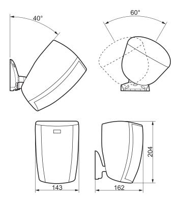
The speaker can be connected to audio lines at constant voltage (100V / 70V) or with constant impedance (8 Ohm).
